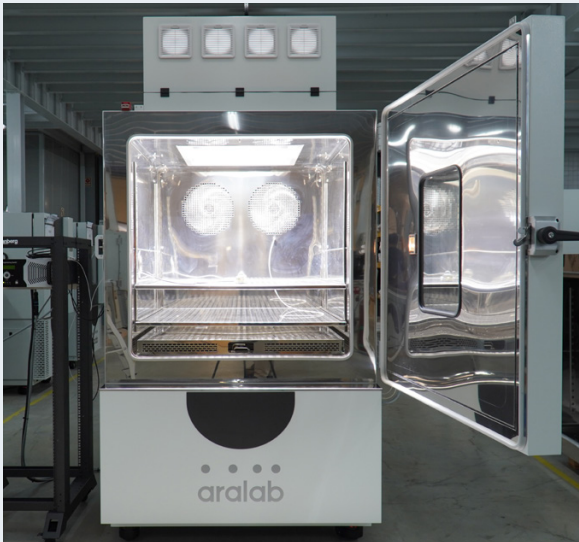
SOLAR AND UV RADIATION CHAMBER
