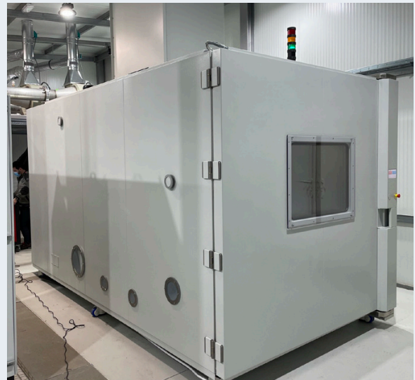
EUCAR ATEX WALK-IN CHAMBERS
